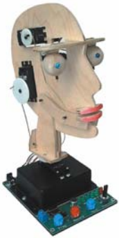
Alex animated head can be programmed from C for PICmicros using the Actuators training panel
